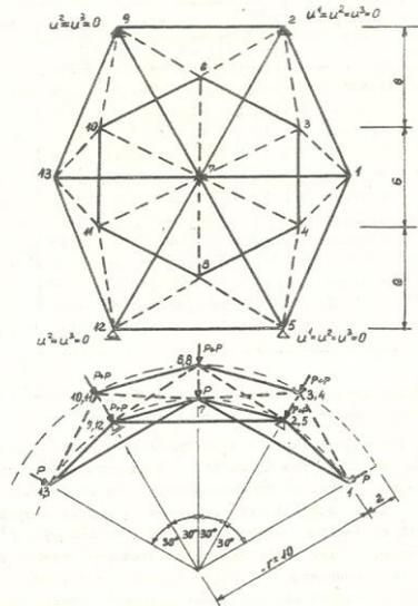
Fig. 34. Double layer hexagonal truss type II; continuous lines means bars in layers, dashed – lines means bracings.
