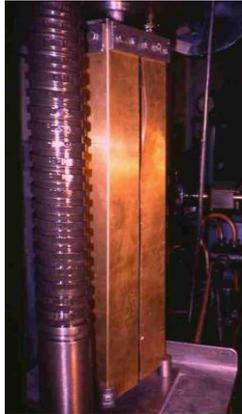
Fig. 12. The specimens, loaded in strength machine; visible three different type waves at free longitudinal edges of slit in middle of wider bar wall
