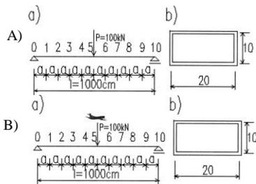
Fig.65. Freely supported steel box beam with moving load Ref 238;  $v=36\text{km/h}$  A)  $v=360\ \text{km/h}$  B).
