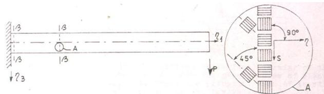
Fig. 5. Cantilever beam and electro-resistance (tissue paper) sensors arrangement (detail A)
