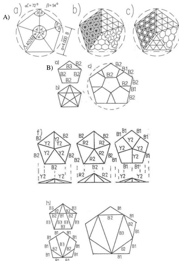
Fig. 57. Possible bar patterns for pentagon, by Zometool elements.
