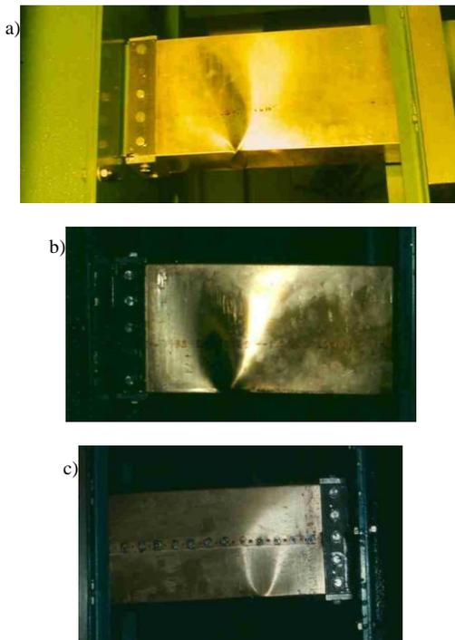
Fig. 7. Cantilever beam with planarly constrained fixed and “free” ends – zones of bimoment influence; a) waves by fastening on side and lower bar walls; b), c) hinge (breaking point) from both sides of bar
