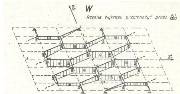
Fig. 27. Deflections of hexagonal band grid should be multiplied by  $\frac{Pl^3}{12EI}$
