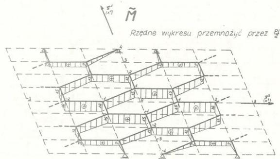
Fig. 28. Bending moments of hexagonal band grid should be multiplied by  $\frac{Pl}{2}$
