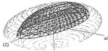
Fig. 74. Scheme of double layer, elliptical space bar structure.
