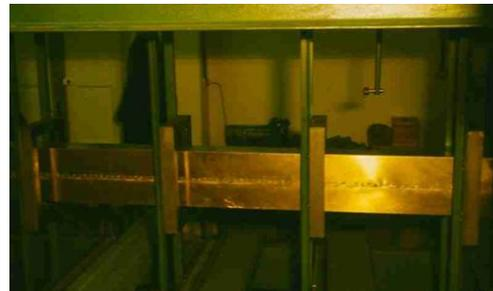
Fig. 3. View on stand for bending-torsion loading of rectangular cantilever brazen beam. Four steel frames helpful by measurements of displacements are visible.
