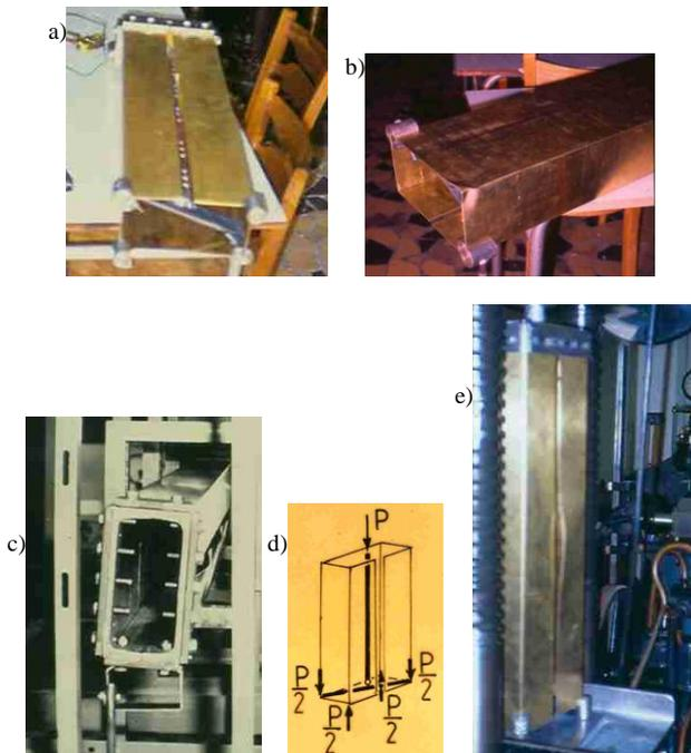
Fig. 10. a,b, d) loading system for bimoment, Visible waves on free longitudinal slits of: c) cantilever (visible strong steel cork); e) of bar loaded by pure bimoment at lower end (four equilibrated forces).
