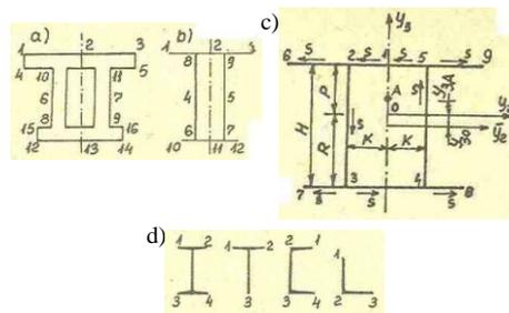
Fig. 70 Types of cross-sections automatically dimensioned in WDKM program system, with shown points for calculation of stresses (compre Fig. 22).
