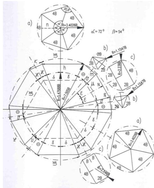
Fig. 55. Detailed geometry of rhombicosidodecahedron.
