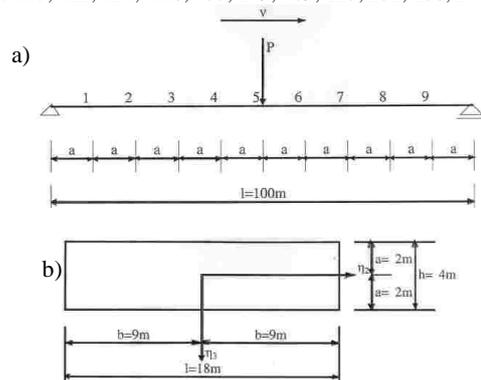
Fig. 63. Scheme of bridge with moving load a), with bridge cross-section b).
