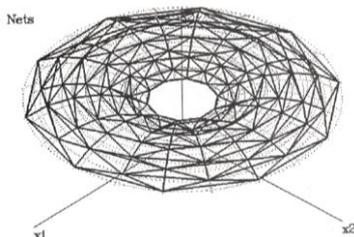
Fig. 71. Single layer space bar structure stretched on torus.
