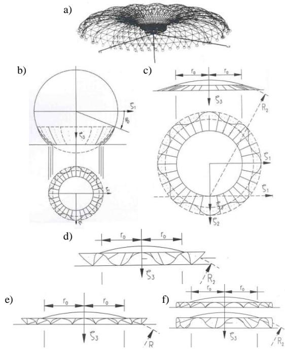
Fig. 52. Examples of wavy space bar structures: a) wavy toroidal, b) wavy supporting part for sphere, c) horizontal waves, d) horizontal-vertical waves, e) absolute horizontal-vertical waves, f) vertical waves. The waves start from certain radius  $r_0$ .
