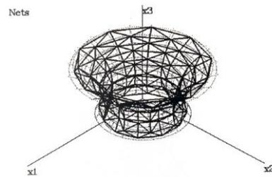
Fig. 72. Single layer space bar structure stretched on torus.
