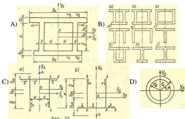
Fig. 22. Types of cross-sections foreseen in WDKM computer system for automatic dimensioning of bars (see Fig 70, too), Ref 11.
