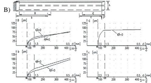
Fig. 8. A) Accordingly to schemes shown in the Fig 4A, the distance of lower part of hinge (breaking point) visible from down for four different cases of the bars with identical wall thickness (0.5mm); B) proper diagrams explaining positions of hinge at lower wall edges.
