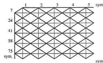
Fig. 79. Double layer truss investigated by B. Zbyszński; nodes – 97-630, unknowns up to – 1890, Ref 262.
