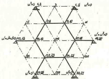
Fig. 32. Double layer hexagonal truss type I; continuous lines means bars in layers, dash & dotted lines means bracings. Underlined numbers are referred to lower nodes.
