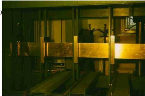
Fig. 6. A) Scheme of optical observation of circuital and longitudinal displacements; B) visible: cantilever beam and steel frames; at left – fastening and hinge (breaking point)
