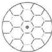
Fig. 47. Maximal regular hexagonal grid inscribed into circle, Ref (4).
