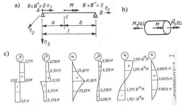
Fig. 35. a) Bar torsioned by concentrated moment; b) central node; c) calculated internal forces.
