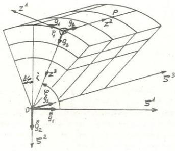
Fig. 23. Definition of cylindrical net of points, Ref 4.
