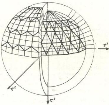
Fig. 25. Example of double layer structure inscribed to spherical net.
