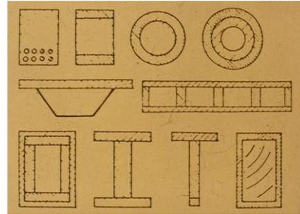
Fig. 18. Different type composite cross-sections
