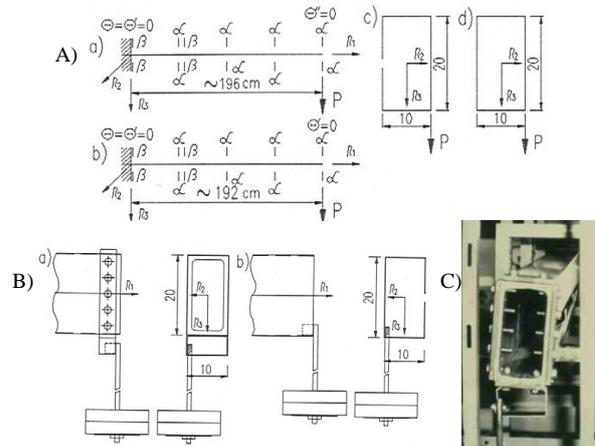
Fig. 4. Scheme of experiment of the Figs 2,3. A) Two applied schemes for cantilever beams: without constrains at free end a) and with planarly constrained displacements b), with rectangular cross-sections: open c) or closed d). B, C) Loading system for thin-walled bars.
