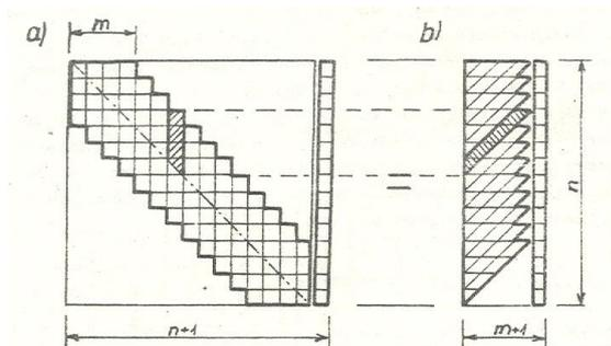
Fig. 67. Scheme of symmetrical set of algebraic equations.
