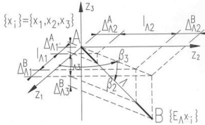
Fig. 54. Definition of angles  $\beta_i$  for bar  $\Lambda$  inclination, (rigid nodes as in the Fig. 21).
