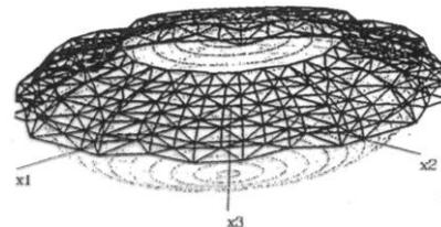
Fig. 75. Scheme of double layer, wavy space bar structure – horizontal waves.
