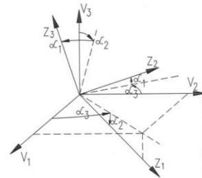
Fig. 53. Definitions of rotation angles between coordinates  $z_i$  - local and  $v_i$  - of support.
