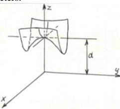
Fig. 69. Definition of the translational nets of points - here as leading global surface is used hyperbolic paraboloid and  $d=z_0+\Delta z$ .
