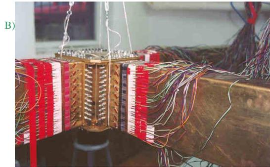
Figure 16. A) Electro-resistance measurements of L type thin-walled frame, with box bars having external dimensions 10x20cm; at the left is visible torsioning moment applied, only; B) electro-resistance measurements of T type of thin-walled frame
