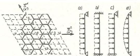
Fig. 26. Hexagonal band plate grid - considered schemes and loadings.
