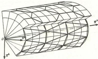
Fig. 24. Example of double layer structure inscribed to cylindrical net.
