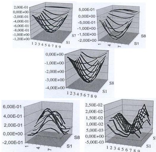
Fig. 64. Diagrams of bridge deflections [cm] under moving load on bridge with span 100m (Fig.63) in eleven time moments (series), with parameters: loading mass  $G=100t$ , loading velocity  $v=36, 180, 360, 720, 3600\text{km/h}$ , bridge mass  $\mu=0.022\ 695\ 016\text{kNs}^2/\text{cm}$ , its rigidity  $EI=2.083\ 333\text{E}+13\ \text{kNcm}^2$ , Refs 240, 241.
