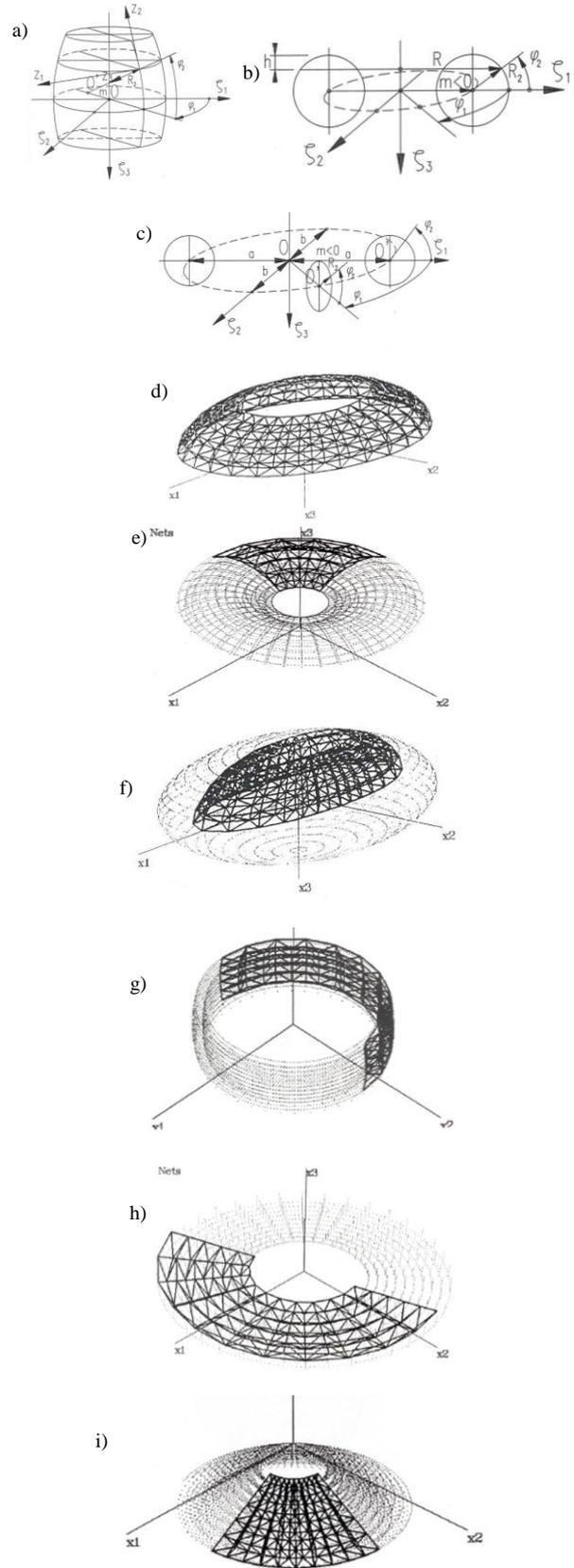
Fig. 51. Definition of nets of points: a) double curvature revolution type; b) toroidal (obtained from case a); c) elliptical (modified net a)); d-i) applications for: double-layer spherical-, toroidal-, elliptical-, barrel-, ring-, and conical type bar structures
