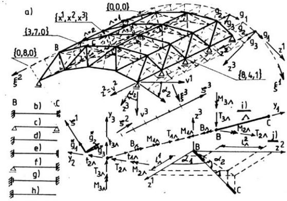
Fig. 46. Definition of more important elements of space bar structures description.
