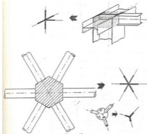
Fig. 21. Nodes with real – „finie dimensions” (see Ref 11 and Fig 55)
