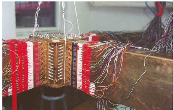
Figure 15. Electro-resistance measurements of T type thin-walled frame with bars having external dimensions 10x20cm.
