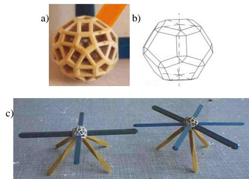
Fig. 59. Geometry of node: a) node used in Zometool kit; b) Rhombicosidodecahedron as a model of node; c) Comparison of the nodes of rectangular and triangular substructures.
