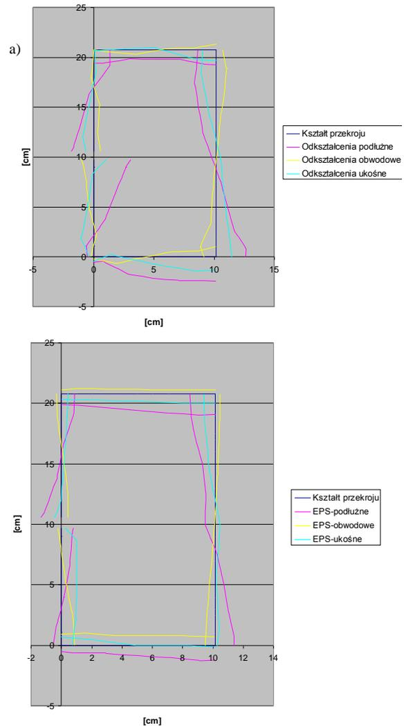
Fig. 17. Diagrams of measured strains for model No 11 with walls thickness app. 1.5 mm, loaded by hanging mass 100 kg; in cross-sections: a) 2 cm and b) 55cm from fastening
