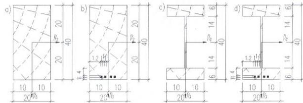
Fig.19. a, d) Homogenous and b, d) composite (reinforced timber) cross-sections
