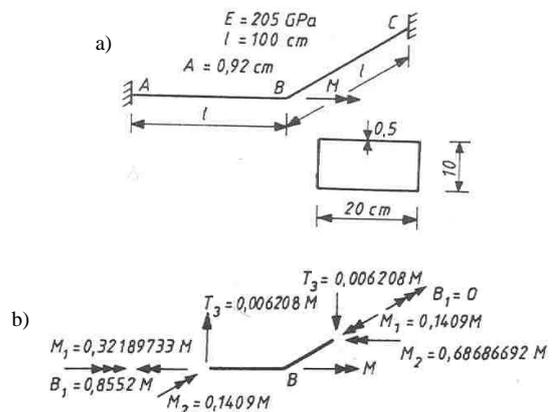
Fig. 36. Plane frame torsioned by concentrated moment, Ref 30.
