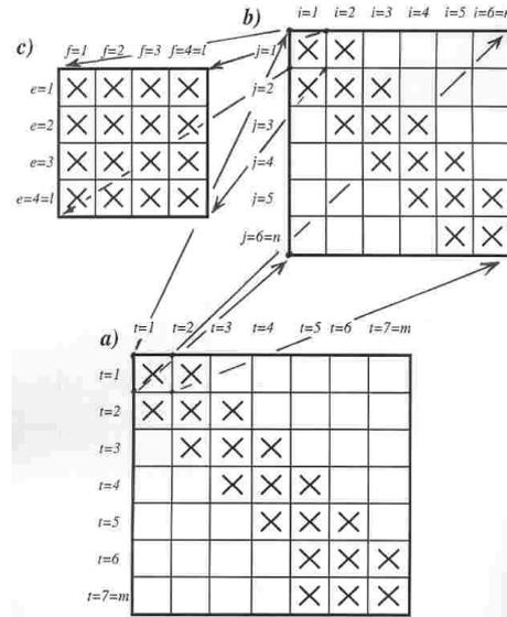
Fig. 62. Detailed scheme of 2D dynamical stiffness matrix for structure considered in 3D-TSM with 6 nodes (b), 4 degrees of freedom per node (c) during 7 time moments (a).
