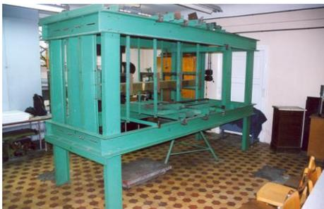
Fig. 2. Stand with brazen cantilever model
