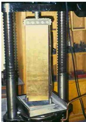
Fig. 13. Visible three different type waves at free longitudinal edges for bars with longitudinal slit on three positions of the wider wall
