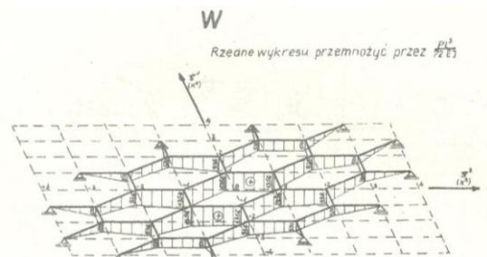
Fig. 30. Deflections for circular grid should be multiplied by  $\frac{Pl^3}{72EI}$
