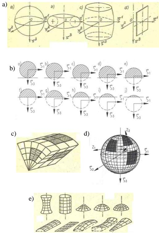
Fig. 49. Possibilities to obtain various architectural effects by: a) choice of global shape of nets of points; b) choosing other parts of spherical net of points; c) d) location of structure on other parts of net of points; e) cutting convenient part of selected nets of points.
