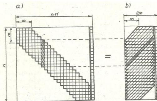
Fig. 66. Scheme of unsymmetrical set of linear algebraic equations.
