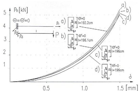
Fig. 9. Capacity of cantilever beams (see Table 1)
