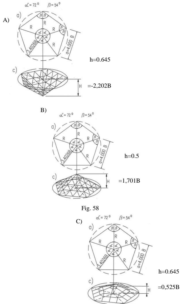
Fig. 58. Global geometry of: A) Concave pentagon with possible bar patterns B) Convex – high possible arrangements by ZOMETOOL elements, C) Convex - low double-layer substructures.
