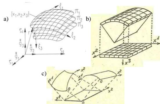
Fig. 48. a)Definition of regular net of points; b) c) transformation of orthogonal coordinates  $x_i$  into curved space (surfaces).
