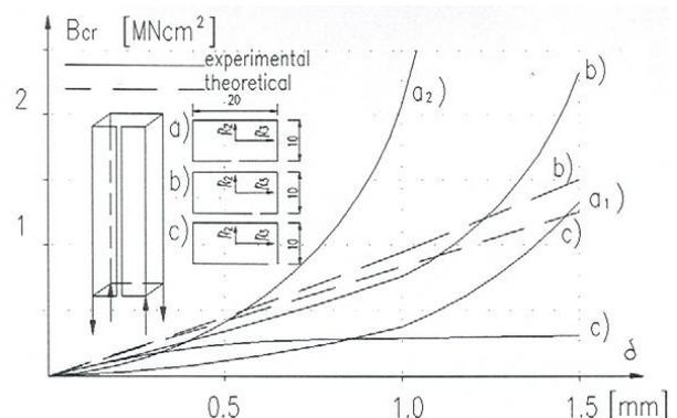
Fig. 11. Observation of critical bimoment (with M.E. El. Awadi, Egypt, Refs 194, 195, 82 (1991, 1992) for short, rectangular bar, with planarly constrained displacements by strong steel cork at top; a), b) loading system by pure bimoment at bottom bar end; c) small damage of supported corner; d) comparison of measured and calculated critical bimoment.
