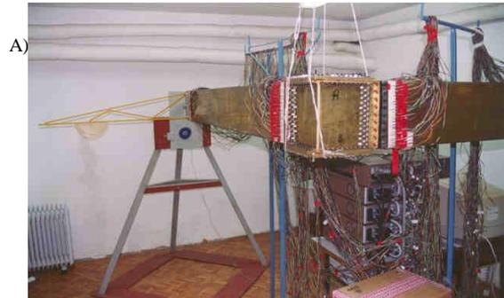
Fig. 14. Frame type L and loading system
