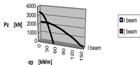
Fig. 37. Ultimate critical curves of forces for simply supported beam with I cross-section (at axes 145.4 and 2161 - lower) and with channel cross-section (at axes 48.559 and 3386 - higher)
