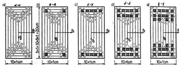
Fig. 20. Cross-sections divided on thin-walled tubes with walls thicknesses 1cm Refs 129, 236 (2000, 2002).
